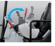
The use of hydraulic pilot type operating levers allows all levers to be securely locked. A neutral engine start mechanism permits engine start only when the lock lever is locked.
