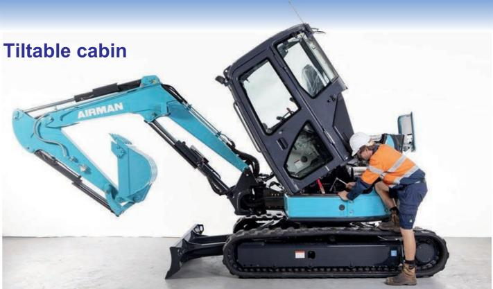
Tiltable cabine allows easy access to the machines main components.
