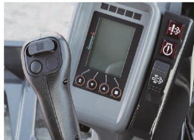
On the AX48U and AX55U-7 the EGR & Muffler Filter system Failure Indicators and the manual regeneration switch are situated next to the monitor.
