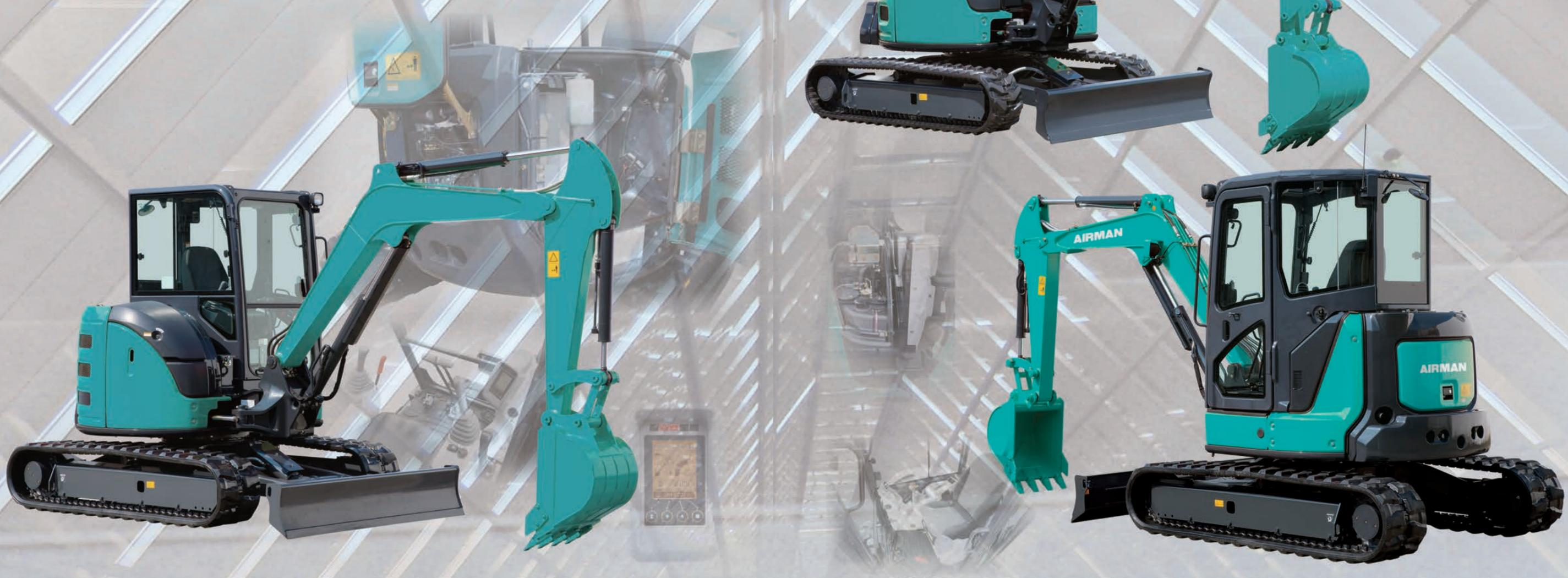
**AX33u-7**    Operating weight **3,330kg**    Capacity **0.08m<sup>3</sup>**
