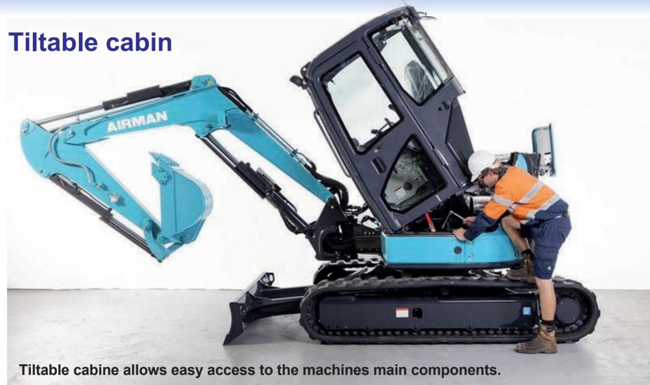
Tiltable cabine allows easy access to the machines main components.
