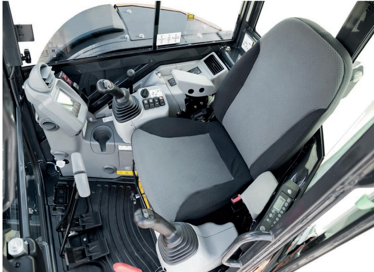
On this specific picture the AX55U-7 full spec machine is visible, equipped with Airco and auxiliary function levers (proportional) to control the attachments.
