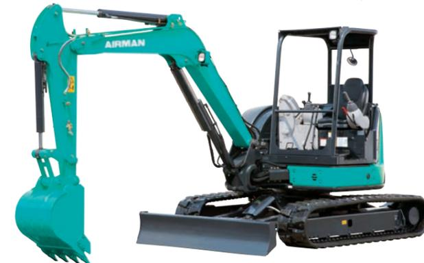
**AX55u-7**    Operating weight **5,210kg**    Capacity **0.14m<sup>3</sup>**
