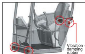
Larger vibration-damping rubber is used in the floor mounts to provide a large improvement in operator comfort.
