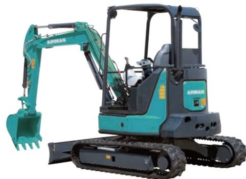
**AX38u-7**    Operating weight **3,960kg**    Capacity **0.10m<sup>3</sup>**
