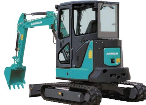
**AX48u-7**    Operating weight **4,770kg**    Capacity **0.11m<sup>3</sup>**
