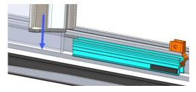
STEP 6: Tilt Panel outward and lift up to remove panel.
