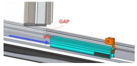
STEP 5: Panel drops to bottom of track which lowers upper edge below frame.
