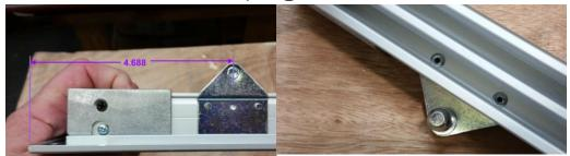
Drill out rivets from inside channel using .1285 drill bit
