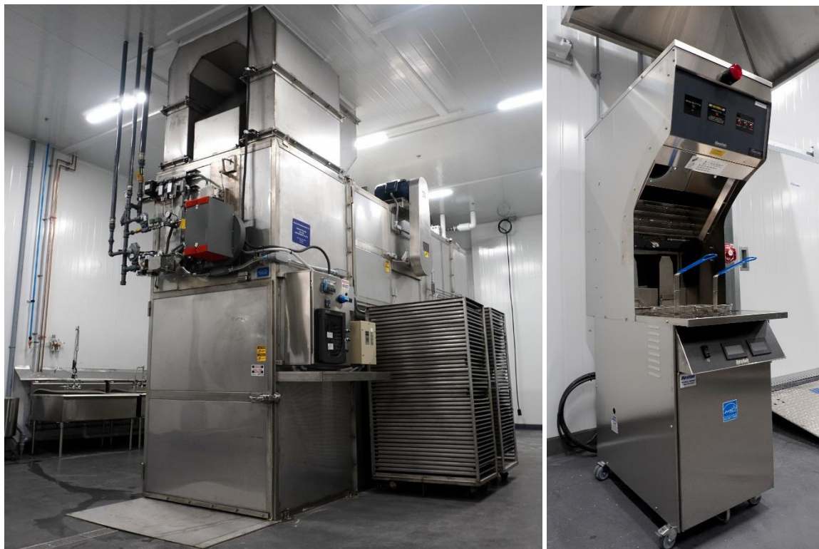
Complimentary food production equipment in REVworx™ including a CDS McKenzie air dryer and fryer
