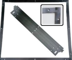
To attach the cut gaskets to the frame surface, solvent activated, or pressure sensitive adhesive systems are applied to one side of the gasket sealing surface. Joints in the dovetail area are typically sealed with RTV materials that are compatible with closed cell sponge polymers.
