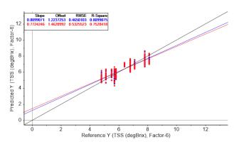
Example Predicted vs Reference plot of the TSS in °Brix for the 12 strawberry samples. The root mean square error of cross-validation tells that the 1sigma error is +/- 0.53 °Brix for each sample.
