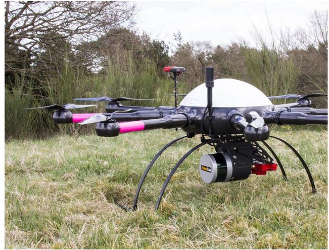
**FIGURE 1** UAS LiDAR system with background of *Cytisus scoparius* shrubs. Photo credit: Urs A. Treier
