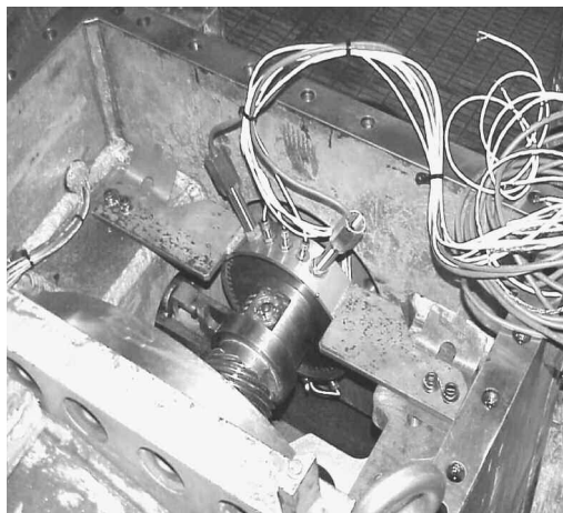
Figure 4. Top Half of Bracket with Sensors Installed.
