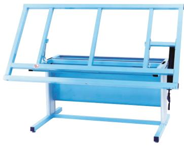
The MWH Manual Height Adjustable Wire Harness assembly benches are designed for the ergonomic assembly of wire harnesses. The unit comes with a 72" x 36" platform capable of holding boards from 24" wide to 24" long up to 48" wide x 96" long. The platform comes with an adjustable front rail that captivates boards from .250" thick to .750" thick. The MWH7236 features a 60 degree 13 position 150 pound capacity tilt. The MWH9636 features a 250 pound capacity.
