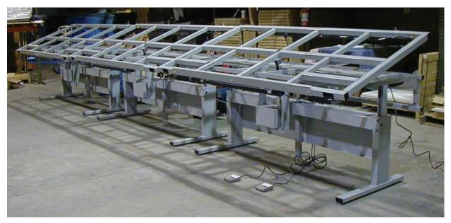
Joinable Wire Harness Station 96" long x 48" deep x 29.250" high when in the flat. Unit adjusts via an electric lead screw. Price includes an 80 degree electric tilt. Both height and tilt adjustment to work via foot pedal. Price includes Master control box that allows benches to be bolted together, any of the connected benches can be designated as master and the balance of the connected benches to work in unison with the master.
