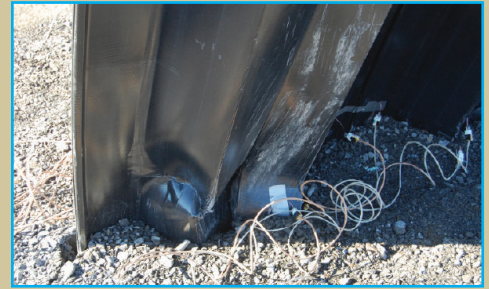
Example of Local Compression Buckling
