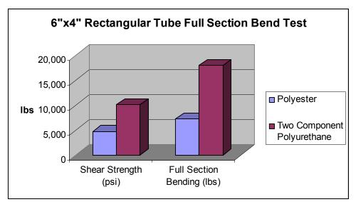
Figure 3.0 Full section bending strength graph
