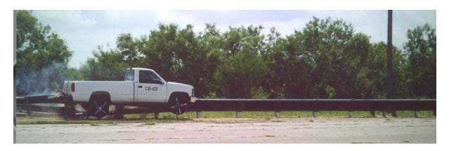
Figure 5.0 <sup>3</sup>/<sub>4</sub> Ton Pickup traveling at 62 Mph; Impact angle 25°
