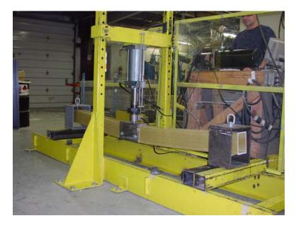
Figure 4.0 Full section bend test
