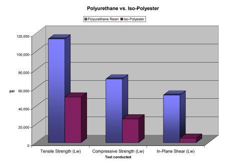
Figure 2.0 Lengthwise mechanical properties
