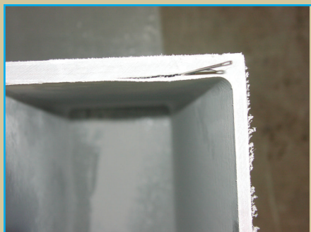
Example of Delamination in a FRP Square Tube
