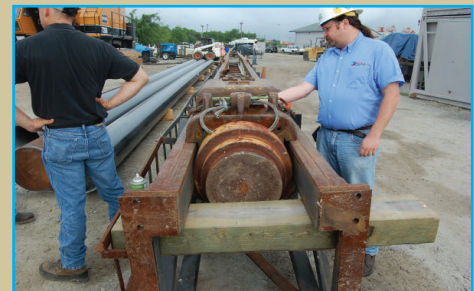
Example of Pipe Insert Driving Head for Driving Hollow Piles
