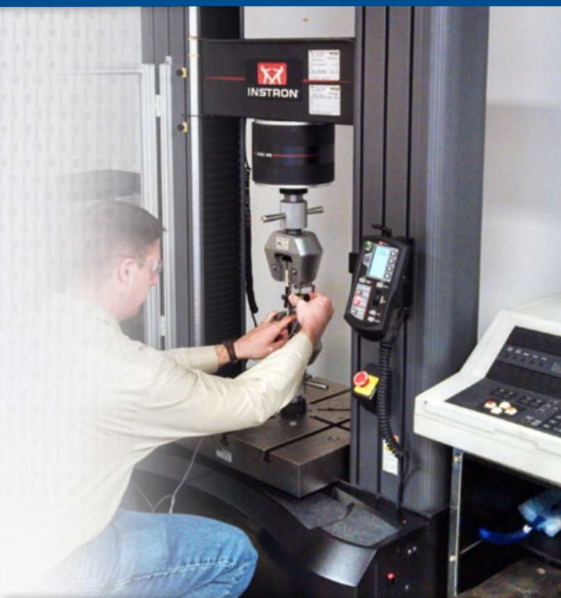
Coupon level tensile testing utilizing CPI calibrated 56 Kip Instron
