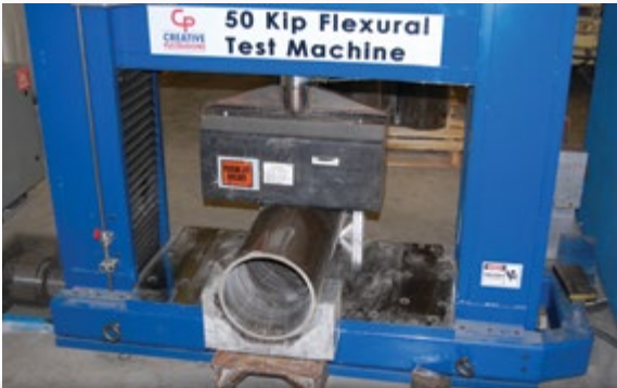
SUPERPILE® Crush Strength Test Set Up
