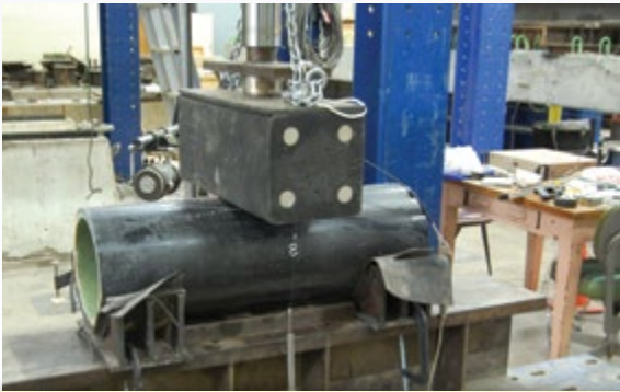
SUPERPILE® with Insert, Crush Strength Test Set Up
