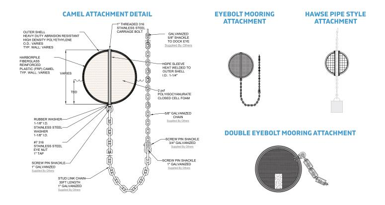
HarborCamels™ feature an abrasion resistant HDPE sleeve, protecting vessels and providing long service life. It has been approved and installed for the U.S. Navy, as well as for customers from Maine to California, to Alaska. Many aspects of the camel can be customized. We can work with you to decide on the best length, diameter, and mooring attachment style for your needs.
