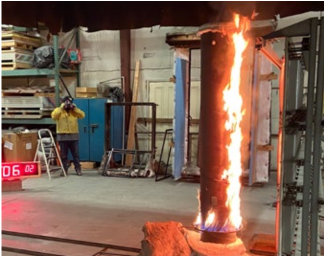
Fire Resistant Pole System being tested for ten minutes at the Western Fire Center.
