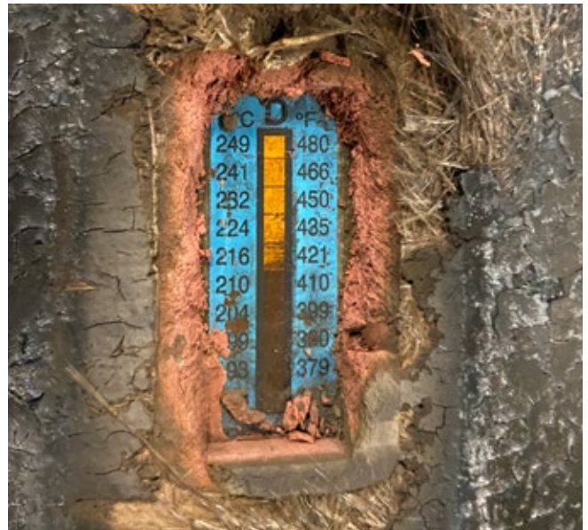
Irreversible Temperature Measuring Device after fire exposure, viewed through the fire protection sleeve.
