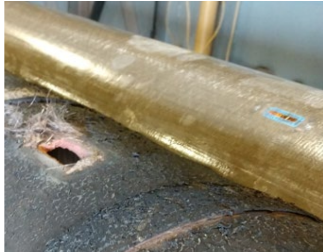
After fire testing, the charred sleeve on the left, and the uncompromised FRP pole on the right.
