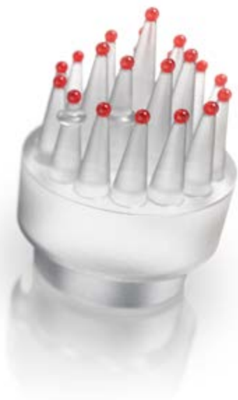
XRM Check: ZEISS has developed a (multi-sphere) length standard for verifying the accuracy of the CT measurements of small-scale dimensions. It is used for determining deviation SD as per VDI/VDE 2630-1.3 guideline.
