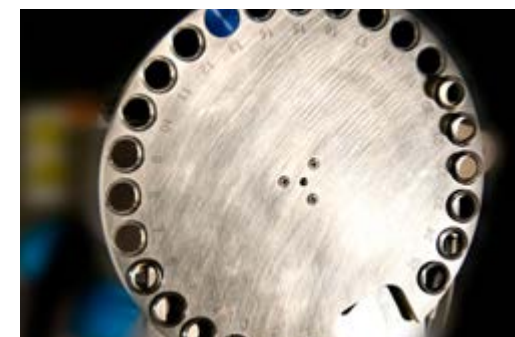
The Automated Filter Changer (AFC) exclusive to the ZEISS Xradia 620 Versa offers 12 standard filters with room for 12 custom filters.
