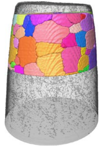
Al 4 Cu alloy showing absorption and grain information. Courtesy of Prof. Masakazu Kobayashi, Toyohashi University of Technology, Japan
