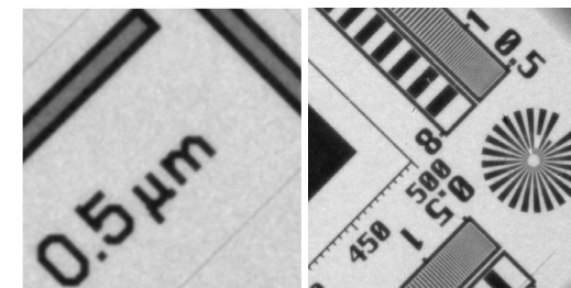
Left: True spatial resolution of 0.5 μm demonstrated on JIMA resolution target Right: True spatial resolution of 0.5 μm demonstrated on ZEISS Xradia resolution target
