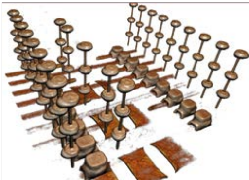
DRAM package interconnect within a 10 mm × 7 mm × 1 mm package containing a 4-die stack. Solder extrusion is easily visualized in 3 dimensions, 0.8 μm/voxel.
