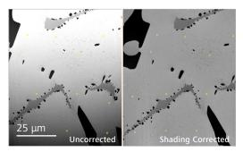
Image filtering: Correct shading, denoise. Nickel carbide alloy imaged by Crossbeam FIB-SEM. Dataset courtesy of P. Bala, AGH University, Poland.
