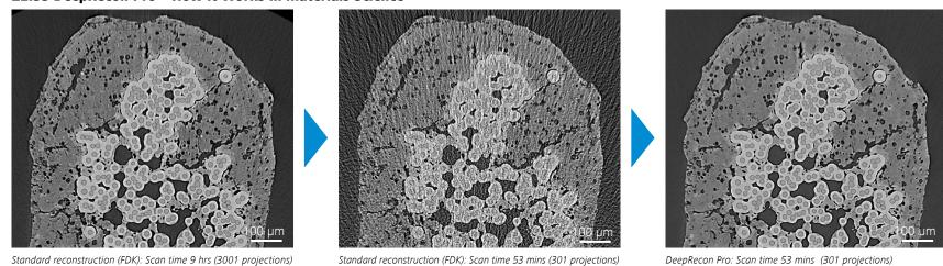
DeepRecon Pro used for throughput improvement for Ceramic Matrix Composite (CMC) sample, achieving 10x throughput improvement without sacrificing image quality. This would allow for much higher temporal resolution for in situ studies.
