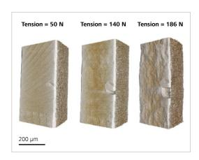
Tensile testing of a steel laser weld under increasing load.
