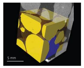
Unstained water in Ottawa sand, imaged in a 12.5 mm diameter aluminum tube
