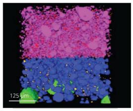
Composite material of polyurethane, EDPM, metal oxides and high melting explosive
