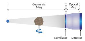
ZEISS XRM Two-stage Magnification Architecture
