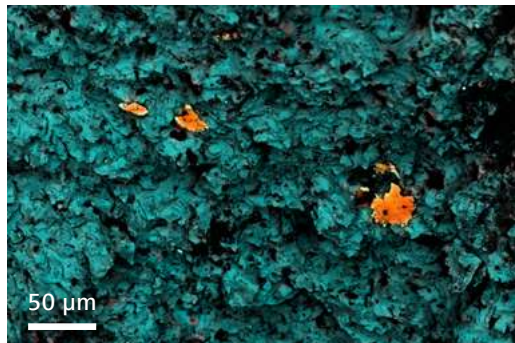
EDS map of fractured sample showing fragments of tin (orange) against the iron (blue) background. Sample: courtesy of J. Scott, West Mill Innovation, UK.
