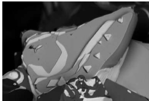
A BiCaCo ceramic is imaged with the low-kV BSE detector at an energy of 5 kV, strong material contrast is delivered by BSEs.
