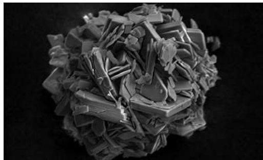
C2D imaging with drastically reduced charging effect
