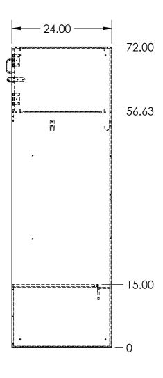
24X24X72 ATHLETIC STRAIGHT VERTICAL VENT LOCKER MADE FROM VARYING THICKNESSES OF FORMICA COMPACT (PHENOLIC) MATERIAL
