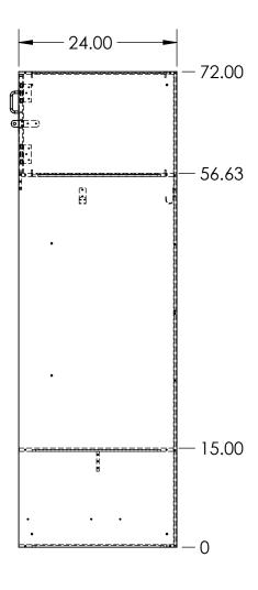
24X24X72 ATHLETIC STRAIGHT OPEN BOTTOM LOCKER MADE FROM VARYING THICKNESSES OF FORMICA COMPACT (PHENOLIC) MATERIAL
