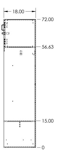
24X18X72 ATHLETIC STRAIGHT OPEN BOTTOM LOCKER MADE FROM VARYING THICKNESSES OF FORMICA COMPACT (PHENOLIC) MATERIAL
