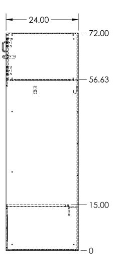
30X24X72 ATHLETIC STRAIGHT MESH GRILL LOCKER MADE FROM VARYING THICKNESSES OF FORMICA COMPACT (PHENOLIC) MATERIAL
