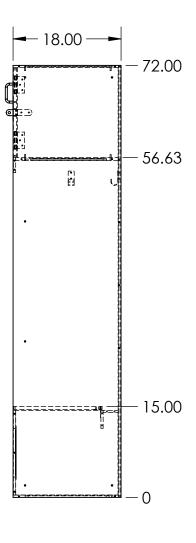
24X18X72 ATHLETIC STRAIGHT MESH GRILL LOCKER MADE FROM VARYING THICKNESSES OF FORMICA COMPACT (PHENOLIC) MATERIAL
