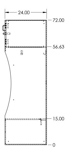
24X24X72 ATHLETIC RECESSED VERTICAL VENT LOCKER MADE FROM VARYING THICKNESSES OF FORMICA COMPACT (PHENOLIC) MATERIAL
