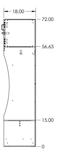
18X18X72 ATHLETIC RECESSED OPEN BOTTOM LOCKER MADE FROM VARYING THICKNESSES OF FORMICA COMPACT (PHENOLIC) MATERIAL
