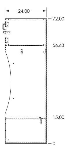
30X24X72 ATHLETIC RECESSED MESH GRILL LOCKER MADE FROM VARYING THICKNESSES OF FORMICA COMPACT (PHENOLIC) MATERIAL
