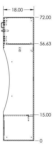
24X18X72 ATHLETIC RECESSED MESH GRILL LOCKER MADE FROM VARYING THICKNESSES OF FORMICA COMPACT (PHENOLIC) MATERIAL
