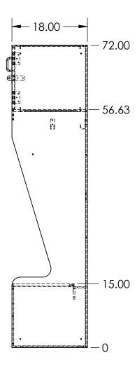
24X18X72 ATHLETIC CUTBACK VERTICAL VENT LOCKER MADE FROM VARYING THICKNESSES OF FORMICA COMPACT (PHENOLIC) MATERIAL
