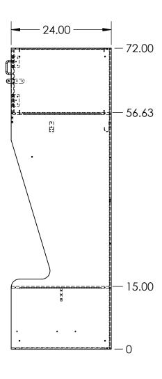
30X24X72 ATHLETIC CUTBACK OPEN BOTTOM LOCKER MADE FROM VARYING THICKNESSES OF FORMICA COMPACT (PHENOLIC) MATERIAL
