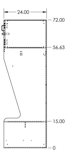
24X24X72 ATHLETIC CUTBACK OPEN BOTTOM LOCKER MADE FROM VARYING THICKNESSES OF FORMICA COMPACT (PHENOLIC) MATERIAL
