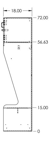
24X18X72 ATHLETIC CUTBACK OPEN BOTTOM LOCKER MADE FROM VARYING THICKNESSES OF FORMICA COMPACT (PHENOLIC) MATERIAL
