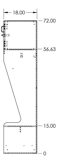
18X18X72 ATHLETIC CUTBACK OPEN BOTTOM LOCKER MADE FROM VARYING THICKNESSES OF FORMICA COMPACT (PHENOLIC) MATERIAL
