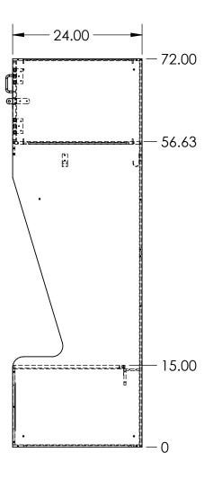
24X24X72 ATHLETIC CUTBACK MESH GRILL LOCKER MADE FROM VARYING THICKNESSES OF FORMICA COMPACT (PHENOLIC) MATERIAL
