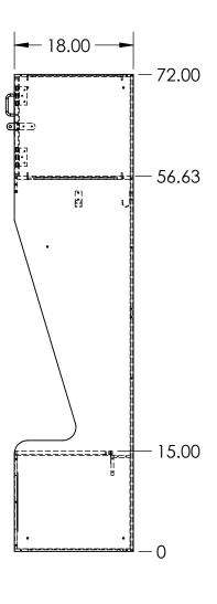
24X18X72 ATHLETIC CUTBACK MESH GRILL LOCKER MADE FROM VARYING THICKNESSES OF FORMICA COMPACT (PHENOLIC) MATERIAL
