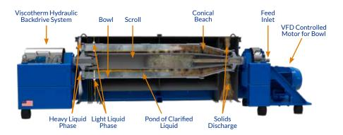
It all starts with a proven performer: advanced hydraulic scroll drive technology. Centrisys replaced the gear box backdrive systems on decanter centrifuges with energy-efficient hydraulic scroll drives from Viscotherm AG in 1988. Today, the Rotodiff® technology saves energy costs for over 2,000 customers worldwide.
