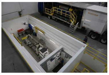
our <u>Centrifuge Balancing Bunker</u>. This dedicated shop space provides the necessary safety and protection of employees and customers who come to witness the operation. It not only provides for noise reduction during high-speed balancing, but it affords a much-needed measure of safety for our operators and service technicians.
