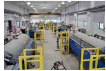
Metro Waster Recovery | Denver, Colorado: Installation is complete for MagPrex, the world's largest struvite recovery installation (from digestate) and (8) CS26-4 dewatering centrifuges.
