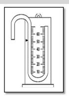
3.4.2. Connect the manometer hose to the plastic valve previously installed in the TSL.
