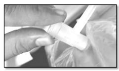
3.4.4. Using a vacuum pump with at least 2.3 cubic meters of suction capacity per minute. Create at least -250 Pascals (Pa) or -25 millimeters' water (mm H<sub>2</sub>O) vacuum inside the TSL by partially opening a portion of the zipper and insert the vacuum pump suction port.
