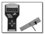
3.6.2. Using the analyzer, carbon dioxide level can be checked through the plastic valve with flexible adapter hose before unloading. Increased carbon dioxide level indicates absence of any source of leaks from punctures, holes or damages. CO<sub>2</sub> level of ambient air is 0.04%.
