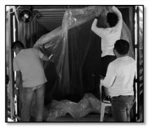
2.1.3. Turn on the ventilator and wait until the TSL spreads perfectly on the sides and ceiling of the container van. A worker can also enter the TSL to help spread the TSL material and help correct any folds in the TSL.
