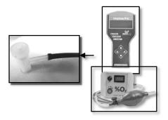
3.5.5. Twist the plastic valve cap to close after taking the readings.
