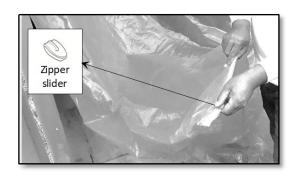
3.3.5. For ease of zipping two persons required, with one person does the zipping and the other person holds the other end steadily making both sections of the zipper in a straight line to avoid the zipper length being misaligned. Moving the slider while the zipper or slider is curved forces one of the zipper sections to elongate.
