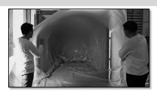
2.1.2. Wait until the TSL spreads perfectly on the sides and ceiling of the container van. A worker can also enter the TSL to help spread the TSL material and help correct any folds in the TSL.
