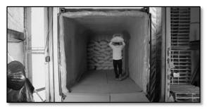
2.1.5. When stacking bags make sure to leave at least 20cm distance between the roof of the container and top of the stacks to prevent condensation.
