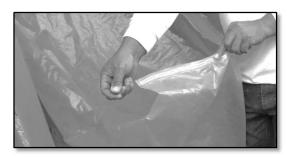
3.3.4. Position the slider on the manually zipped portion of the zip lock.
