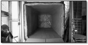
2.1.4.1. **For Manual Loading -** workers should not wear shoes with spikes that might cause damage to the liner.
