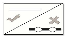
3.3.7. Fold extra liner and tape it against the stack. Ensure that no liner is stuck in-between doors.
