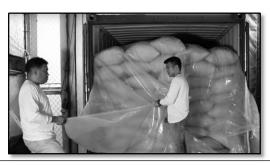
3.3.7. If uneven zipper ends are observed, slightly stretched and redo the zipping from end to end.
