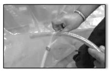
4.3.5. Open a section of the zipper and insert the pressure kit. This serves as outlet to discharge  $O_2$  when flushing.
