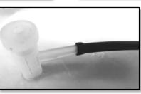
3.4.3. Twist the plastic valve cap to open.
