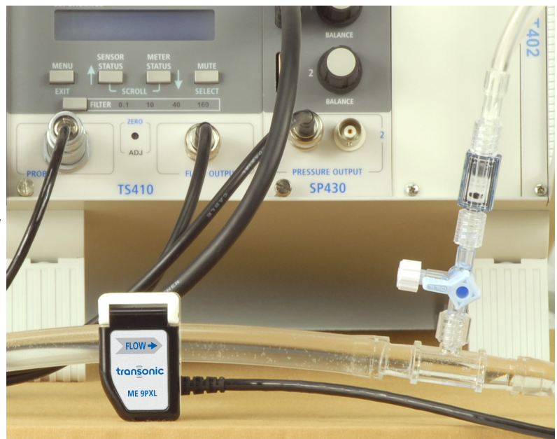
MEnPXL Clamp-on Flowsensor and external pressure sensors on mock circulatory loop.
