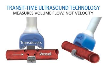
Two transducers pass ultrasonic signals, alternately intersecting the vessel in upstream and downstream directions. The difference between the two transit times yields a measure of volume flow.
