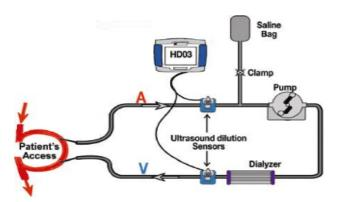
Fig. 1: Transit-time flow/dilution sensing during hemodialysis.
