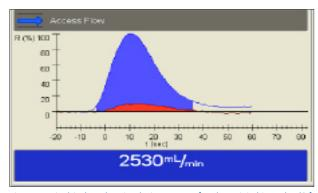
Fig. 6: Typical induced recirculation curves for the Krivitski Method® for calculating Qa.
