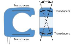
COnfidence Flowprobes<sup>®</sup> use four transducers to create an X-beam ultrasonic illumination pattern to achieve a full vessel volume flow measurement.
