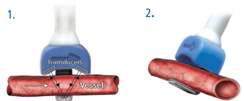
Figs. 1,2: Front and side view of optimum vessel positioning within the ultrasonic window of a Transonic Microvascular Flowprobe.
