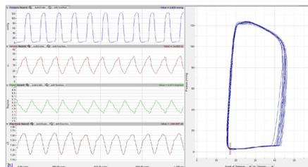
Admittance method measure pressure, volume, phase and magnitude in real-time, creating pressure-volume loops.
