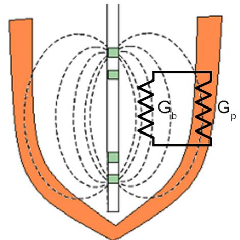
Conductance uses a circuit model where both blood ( $G_b$ ) and cardiac muscle ( $G_m$ ) are conductive and measured together as a single conductance value ( $G_x$ ) and phase components are ignored.
