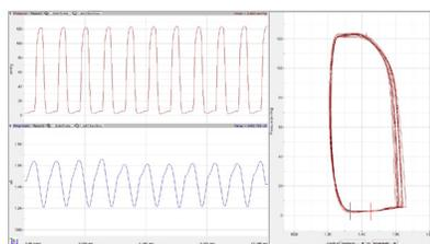
Conductance method measure pressure and magnitude in real-time, creating pressure-magnitude loops. Volume can only be calculated post-experiment.
