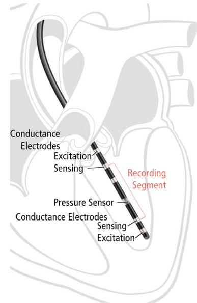
Conductance excitation electrodes create an electric field while sensing electrodes measure the voltage change which allows for the calculation of resistance and conductance.
