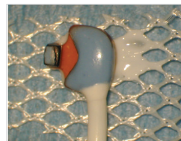
Fig. 4: A 0.5PSS Flowprobe prepared with dacron mesh attached to the underside of the Probe with silicone adhesive.
