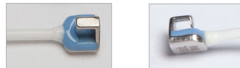
Fig 3: 1.5PSL Probes are designed specifically for chronic implantation on the ascending aorta of the mouse. The transducer housing is less than 5 mm and is easily accommodated in the mouse thoracic cavity. The non-constrictive fit does not interfere with the ascending aorta or pulmonary artery. For connector exteriorization, the Probe's flexible cable is tunneled under the skin.
